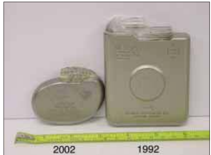
Changes in implantable cardioverter defibrillators over 10 years (1992-2002). Apart from the marked reduction in size, the implant technique and required hardware have also dramatically improved—from the sternotomy approach with four leads and abdominal implantation to the present two-lead transvenous endocardial approach that is no more invasive than a pacemaker implant
